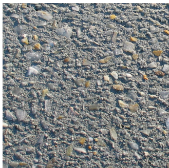
Insitu Exposed Aggregate Concrete PEDESTRIAN PAVING
