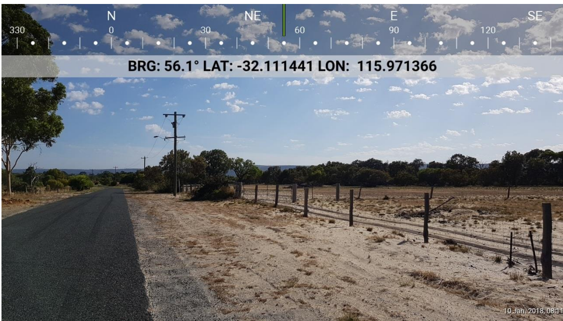
Photo 22: Low threat and non-vegetated areas excluded from classification under Clauses 2.2.3.2 (e) and (f) of AS 3959 on left; Class G grassland and Class B woodland on right
