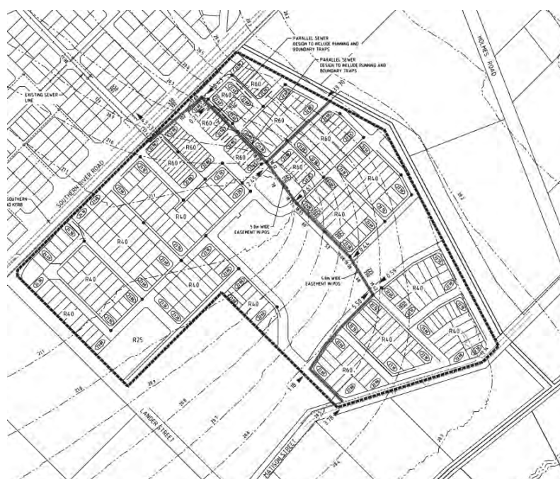
Figure 6 – Water Corporation Multi-Stage Works Agreement Sewer Planning
