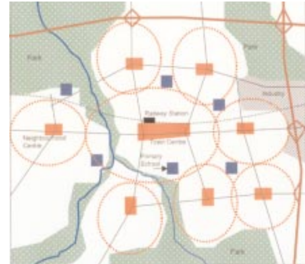
Fig 6. Desirable urban structure. Neighbourhoods defined by five-minute walking distance (400 metres) from a neighbourhood centre, with net residential density of 30-80 dwellings/ha, clustered around a town centre with railway station. Neighbourhoods are linked directly to each other and with the town centre. Primary schools are located to facilitate easy, safe access, and are “shared” between several neighbourhoods. Large industrial areas, and other large land users are ideally located at the edge of the town or neighbourhood.
