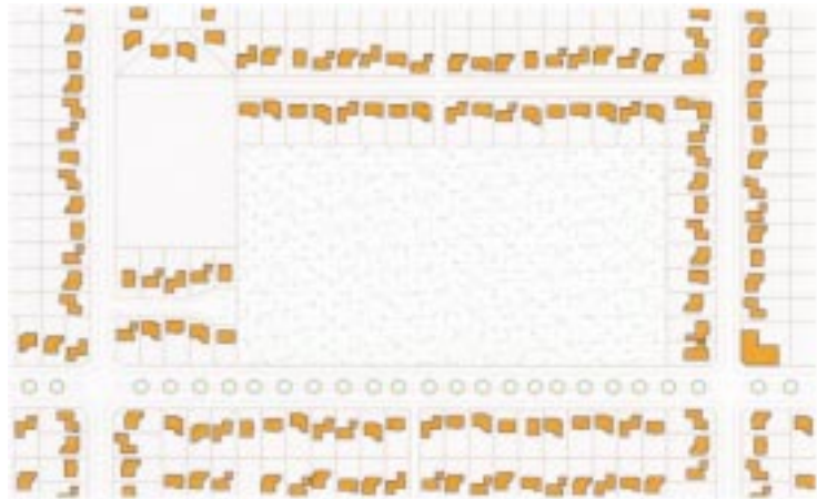
Fig 25. An example of the redesign of a park to achieve better safety outcomes. The park has houses “backing onto” the park with high fences facing the park. This condition achieves poor levels of safety in both the houses and park. The redesign introduces new houses, which face the park, creating safety in the houses and in the new park. Streets have been connected to provide safe access to the park from surrounding areas.
