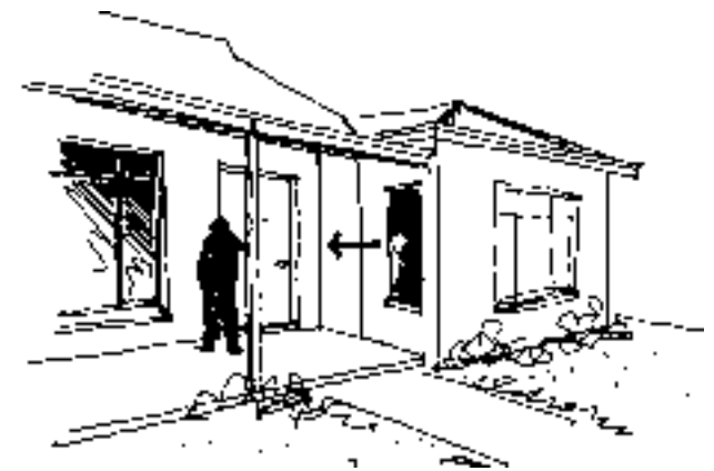
Fig 32. Design and locate windows to increase surveillance, especially of doors and other points of access.
