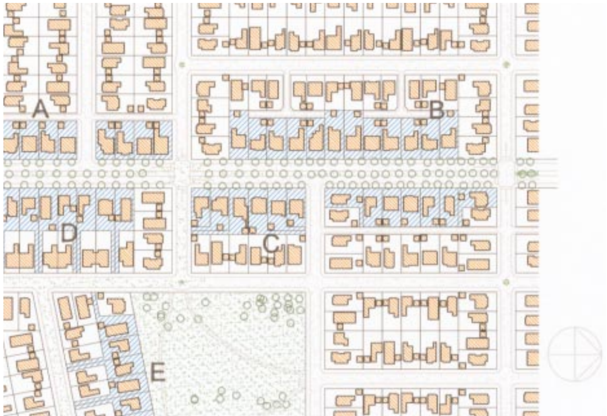
Fig 21. This diagram shows a number of techniques which can be used to achieve frontage and vehicle access in difficult circumstances. (A) rear lane access, (B) reciprocal right of way, (C) battle-axe lots entering from a side street, (D) battle-axe lots entering from a back street, (E) battle axe lots facing a park. This should only be done when the lots facing the park are also north-facing, to avoid high walls fronting the park.
