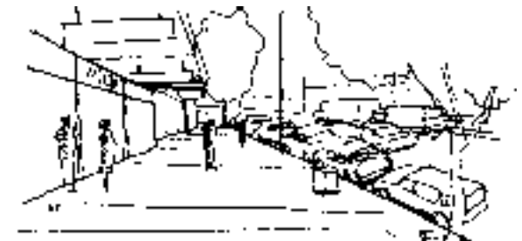
Fig 13. On-street parking as a “barrier of steel” protecting pedestrians.
