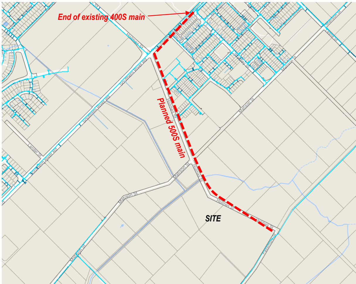
Figure 9: Required Distribution Mains Extension
