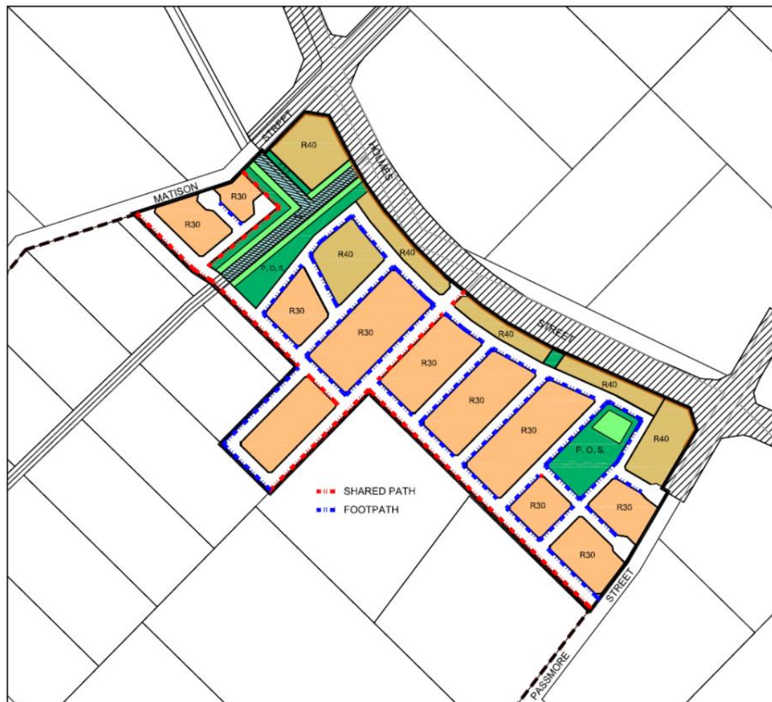
Figure 14 – Recommended Path Network
